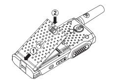
3 Slide battery latch into lock position.
