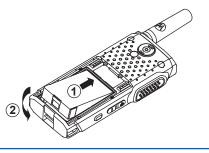
2 To attach battery cover, align it in place and slide the battery latch until it snaps into place.
