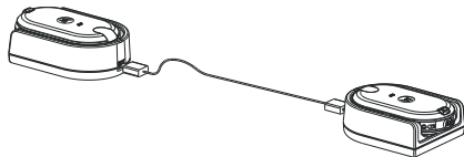
Klona radion via en SUC-laddare (Single Unit Charger)
